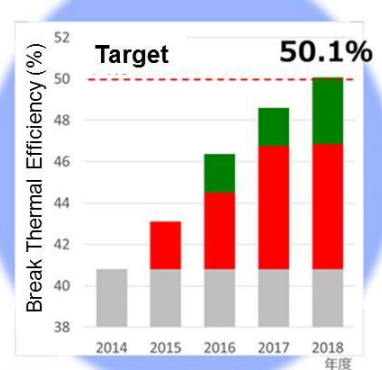
Fig. 2: Improvement of Maximum Break Thermal Efficiency
