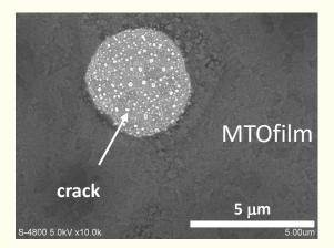
Fig. 1 Surface morphology of magnesium-tin oxide (MTO) film
