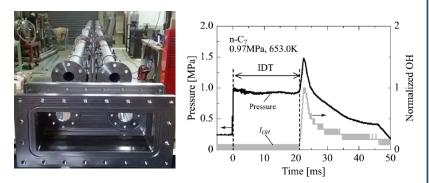
experimental and numerical results. Fig. 1. Appearance of shock tube facility (left) and IDT of  $n-C_7H_{16}$ .
