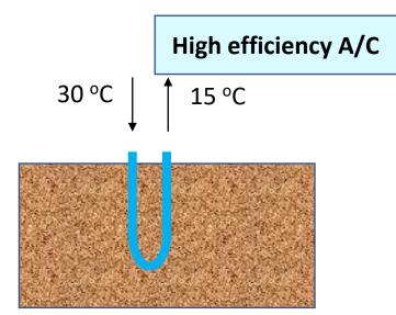
\*Underground temperature is constant throughout year. It can supply cold water when hot, and hot water when cold to achieve high efficiency of air conditioner.
