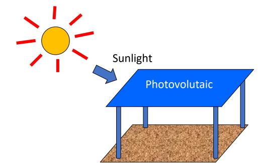
\*Solar sharing is to put roofs over part of the farmland so that both agriculture and solar power generation is made simultaneously.
