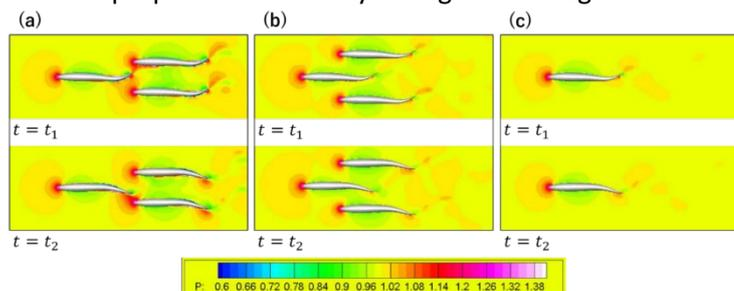
Fig. 2 Pressure Variation (a)  $S=1.0L, B=0.2L$ , (b)  $S=0.5L, B=0.3L$ , (c) Single Fish
